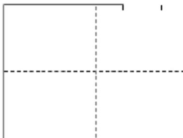
**Fig. 1: Line off entire area to be installed.**
